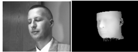
Figure 1: Two different views of RK. On the left is a video image. On the right is a depth map of a model of RK that describes the distance to each of the visible points of the model. Closer points are rendered brighter than more distant ones.
