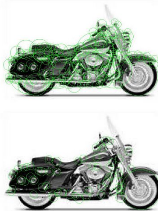
Figure 1. Output of the Kadir-Brady feature detector with different parameter settings. The circles represent the locations and scales of salient regions.
