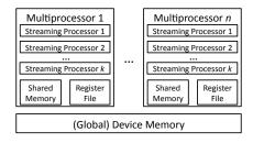
Figure 5. Simplified GPU hardware architecture.
