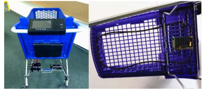
Figure 4: The intelligent shopping card: The handle of this shopping cart is fitted with a 7 inch touch screen, a finger print scanner and a single button (photograph taken from the back, left). An RFID antenna is placed under the product basket to recognize which products are placed inside the cart (from below, right).
