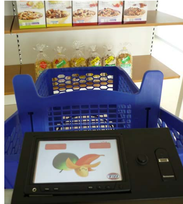
Figure 1: The interactive shopping card attached to the handle bar of the intelligent shopping car.
