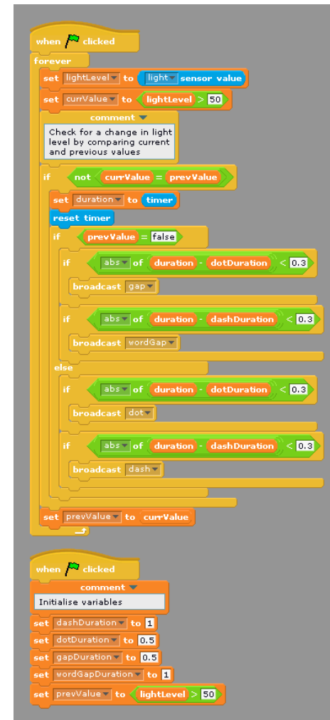
Figure 1. An example of a Sense program showing how program structure is made clear using different shaped blocks and colour.
