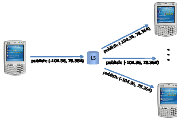
Figure 2. The device on the left has delegated its location subscriptions to a proxying locations service, "LS", shedding network load.
